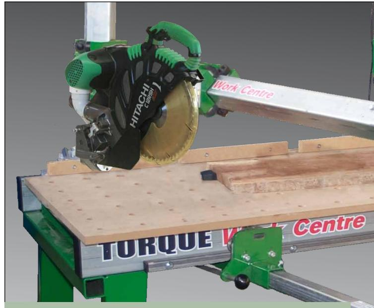
Whether it is a hobbyist's shed, or a production workshop, the Torque Workcentre quickly becomes an indispensable tool. Having a router mounted overhead turns a 7kg handheld router into a 157kg powerful, versatile machine. A circular saw becomes a radial arm saw, or a sliding compound mitre saw with up to a 1300mm cut. A drill becomes a drill press with phenomenal reach away from the drill press pillar.
