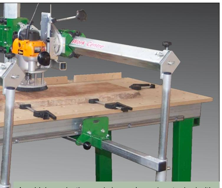
In a high-production workshop, a large 4 metre bed with dual (or triple) carriages for rapid tool changes allowing multiple machining steps to be executed quickly and accurately.
