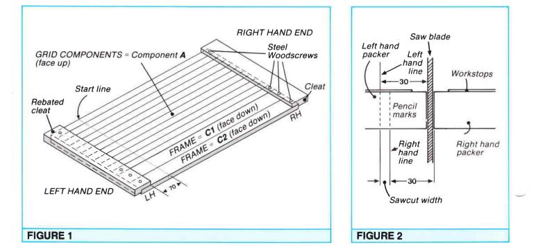
Convert to the crosscut mode and ensure that your saw is cutting squarely. Using a length gauge on your workstops cut all the material to 900mm lengths, saving the offcuts.
