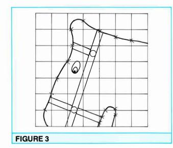
Round over both sides of the legs, seat, head, handle support and the sides of the uprights, components L, M, N, O, G and A. Don't round over any edges that butt up to other components, for example, the tops and bottoms of the uprights A, the tops/bottoms of the legs L, M etc.
