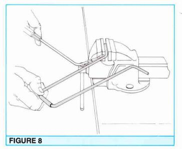
Try to keep the shape of the bracket as close as possible to that in **Figure 1**. The use of a small oxy-acetylene torch (most L.P. gas torches are not hot enough) helps in achieving tight, sharp bends. Repeat the above procedures for the second bracket. It is important that the bushes **R** move freely on the brackets to allow the horse to swing smoothly.
