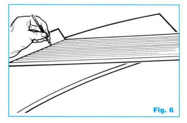
Lay the two reinforcement braces (E) diagonally across the back of each arch, in the positions shown in Fig. 6 & 7. If your decking boards have a grooved side, ensure the smooth side is against the arch. Mark upper and lower cut lines on each brace at the edges of the arch. Number your braces and the arches to identify their location when re-fitting.
