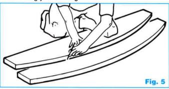
Along the bottom edge on the "OUT" side of one of the arches make a pencil mark 200mm in from the left and from the right. Place the other arch on top ("OUT" sides together) and position it so that the cut curve begins and ends at the two pencil marks and the ends line up. Trace your lower curve onto the arch. **Fig. 5**
