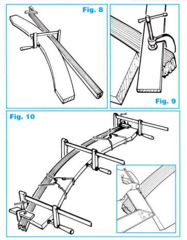
Rest a straight edge against the ends of the arch and mark a vertical pencil line at each end of the hand-rail as a cutting line for the ends of the hand-rail. **Fig. 10 Inset.**
