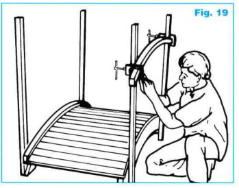
Ensure your posts are square to the ground then trace the curve of the hand-rail onto the post to create your cutting line. Mark a line on the underside of the hand-rail on either side of each post to identify where to position the corner brackets. **Fig. 20**
