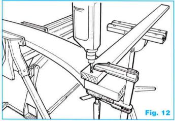
Finger tighten the Coach Bolts, washers and nuts through the holes to fasten the post into position. **Note:** 4" bolt in the top hole and  $4^{1}/_{2}$ " in the bottom. Repeat the above procedure with the remaining three posts.
