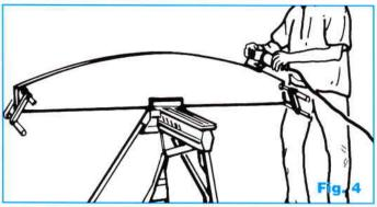
Clamp the two arches together ("OUT" sides facing each another) and sand the two curves evenly. **Fig. 4** Using a coarse grit on a Triton Random Orbital Sander made light work of this otherwise laborious task. Depending on the quality of your jigsaw cuts and the availability of an aggressive sander you may need to plane them before commencing your sanding.
