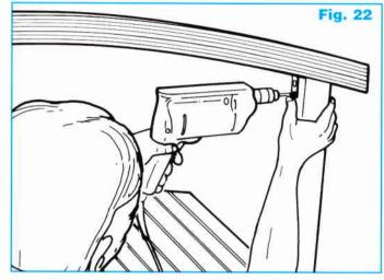
Remove the hand-rails, apply Liquid Nails (or similar) to the tops of each post. Re-locate the handrail and screw into position. Fig. 22 Wipe away any excess glue.
