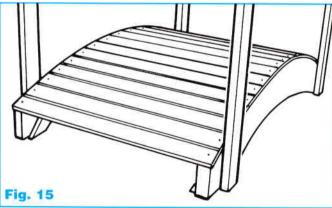
Drill 3.5mm holes into the arch, using the treads as templates and lightly screw each into position using 50mm countersunk screws. Start with each of the end treads first and work in towards the centre using your spacer each time - check for squareness as you go. Continue this procedure until you have 4 - 5 treads left in the centre. **Fig. 16**
