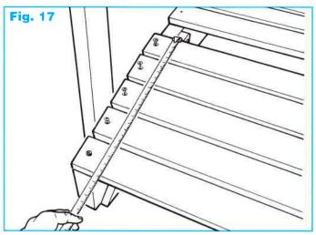
Lay your last 4 - 5 treads across the remaining gap then drill and screw them evenly into position compensating for any gap discrepancies. **Fig. 17**
