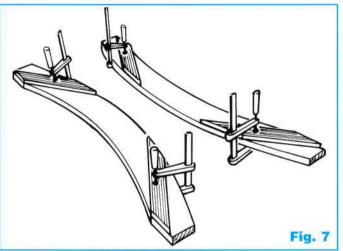
Mix up some Hard & Fast Woodworking Adhesive (or similar), wipe clean your workpieces then glue and clamp the braces into position. **Fig. 7**
