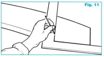
Drill two 8mm holes 20mm & 130mm up from the bottom of each post (D). Clamp the handrail support to the outside of the line on your arch, ensuring it is flush with the base of the arch and level with your line. Use the two holes as a template to drill through the arch **Fig. 12** As you will be drilling through three sections of material you may need to drill as far as your bit will allow, then remove the post to complete the drilling.
