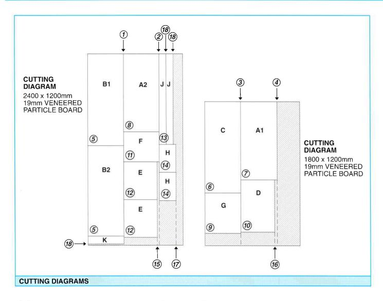
Make trenches 19mm wide and 9.5mm deep across the full width of components A, B, C, F, and G. Turn the pieces as necessary for ease of working, and align your previously marked lines with the appropriate side of the sighting notch in the front fence. (Figure 2). It is best to take several cuts to reach the full depth of each trench, rather than one deep cut of 9.5mm.
