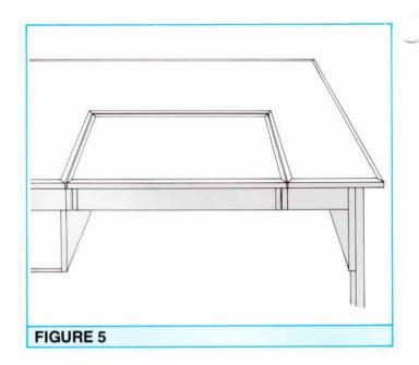
Cut O to size. On your desk top, measure to the centreline of the slot from the front edge of the desk. Mark the centreline parallel to the front and slightly longer than **O**. Mark out the centreline on **O** as well, place in position on the desk top, and use a sharp pencil to scribe around **O**. The slot should also be central to the shelf unit.
