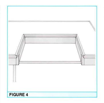
The back panel is attached to the side panels by means of particle board screws. It is further strengthened by the addition of a long corner block that runs along the inside join of the top and back panels. Cut this from your 19 × 19mm material, and screw into place, taking care not to drill or screw through either the top or the back panel.
