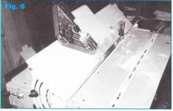
Change the Guide angle to 50°, flip the wall panels around and bevel cut their tops (one of their long edges) for the roof panels to attach into. Using the protractor makes it easier to support the wood as it is cut (**Fig. 7**).
