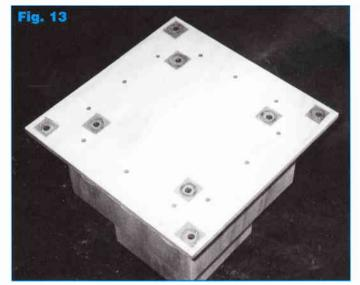
Drill pilot holes, approximately 45mm in from the edges of the bottom level base, ensuring the wall section is centred on the base. Glue and screw it to the base level walls using twelve 25mm treated pine screws. Three into each wall (**Fig. 13**).
