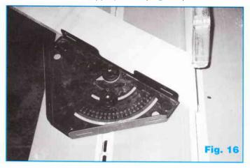
Mitre cut one end of the other two pieces but this time set the protractor to 12.3° using the same scale. This will create two "corners".
