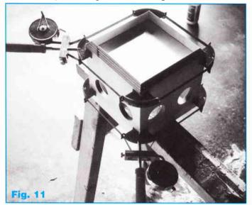
We used two web clamps for this job (**Fig. 11**). They are terrific devices, traditionally used for clamping picture frames together but great for lots of other gluing jobs. They have a steel web and four corner blocks. As the clamp is tightened the web becomes taught and hold the blocks against the workpieces drawing them evenly together.
