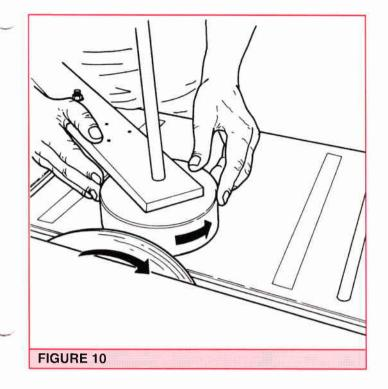
Do not tighten the clamping nut fully yet. Place a wheel in position, insert the axle and make sure it goes into the bottom hole. The wheel should turn freely on the axle. Slide the jig in the table slot until the wheel meets the sanding disc at a fairly steep angle, and in the middle (highest point) of the sanding disc, then lightly tighten the nut so that the jig is held firmly but is still free to pivot.
