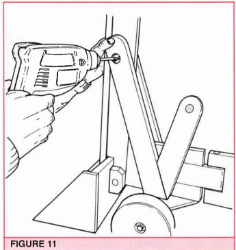
Remove the bucket assembly and drill the hole in the bucket arm (L) for the dowel axle. The bucket arm should pivot freely on the axle, and when satisfied cut the dowel to length and fit the bucket assembly, pinning the axle in place with two screws through the front of the support arms (K). 30mm I.D. steel washers are placed wither side of the bucket arm to centralise it in the gap between the support arms.
