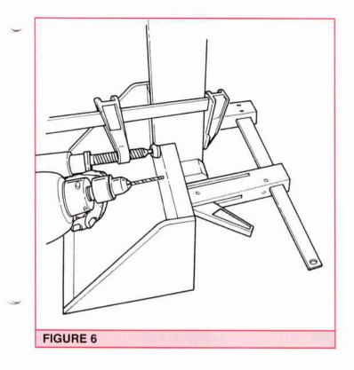
Cut the dowel pivot the length and drill and fix it in place with the fixing screws. Make sure the bucket pivots freely; you may need to take out the dowel and further round the lower end of the bucket arm to give greater clearance. Too small a clearance at this point will lead to sand grains jamming in the gap and interfering with the pivot action. Fit a bump rubber stop, if desired, to the lower back (N) of the bucket.
